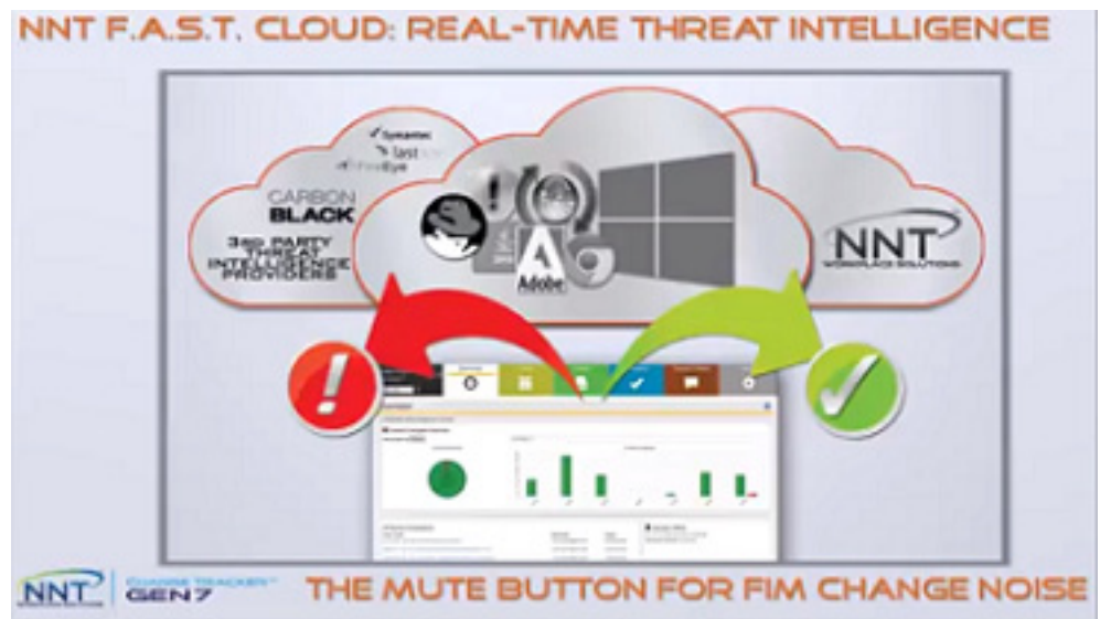
Figure 1: NNT FAST Cloud leverages external threat intelligence and whitelisted facilities to automatically approve the validity of File Changes as they occur.
